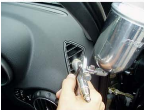
The machine sprays a fine mist of titanium dioxide in the cabin.
